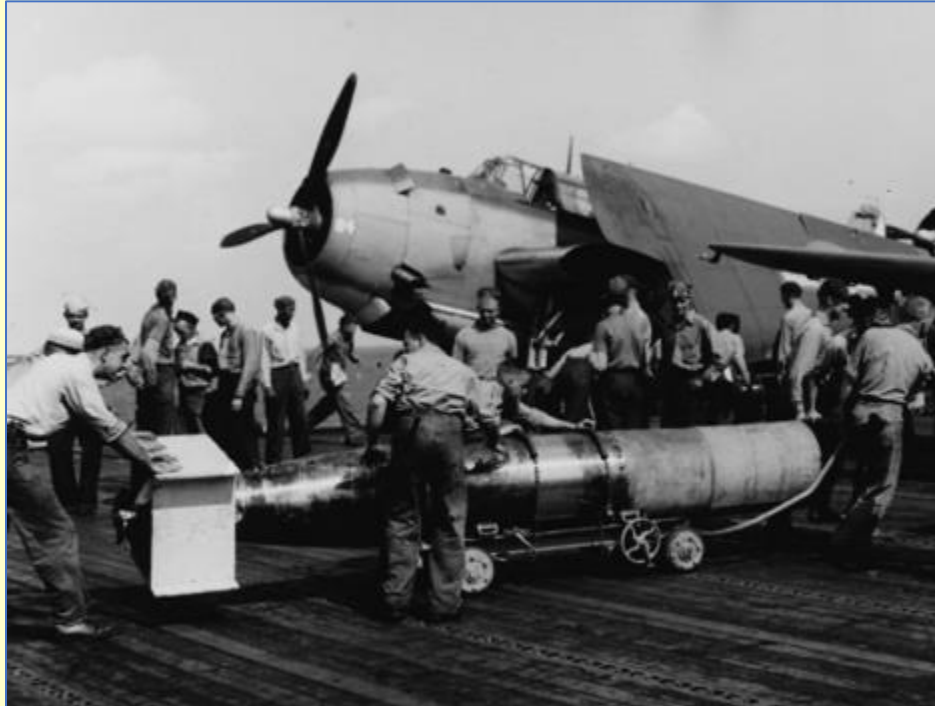
A Mark 13 with drag ring and stabilizer, but no the shroud ring being loaded onto a TBF on board the Wasp (CV-18) October 1944.
