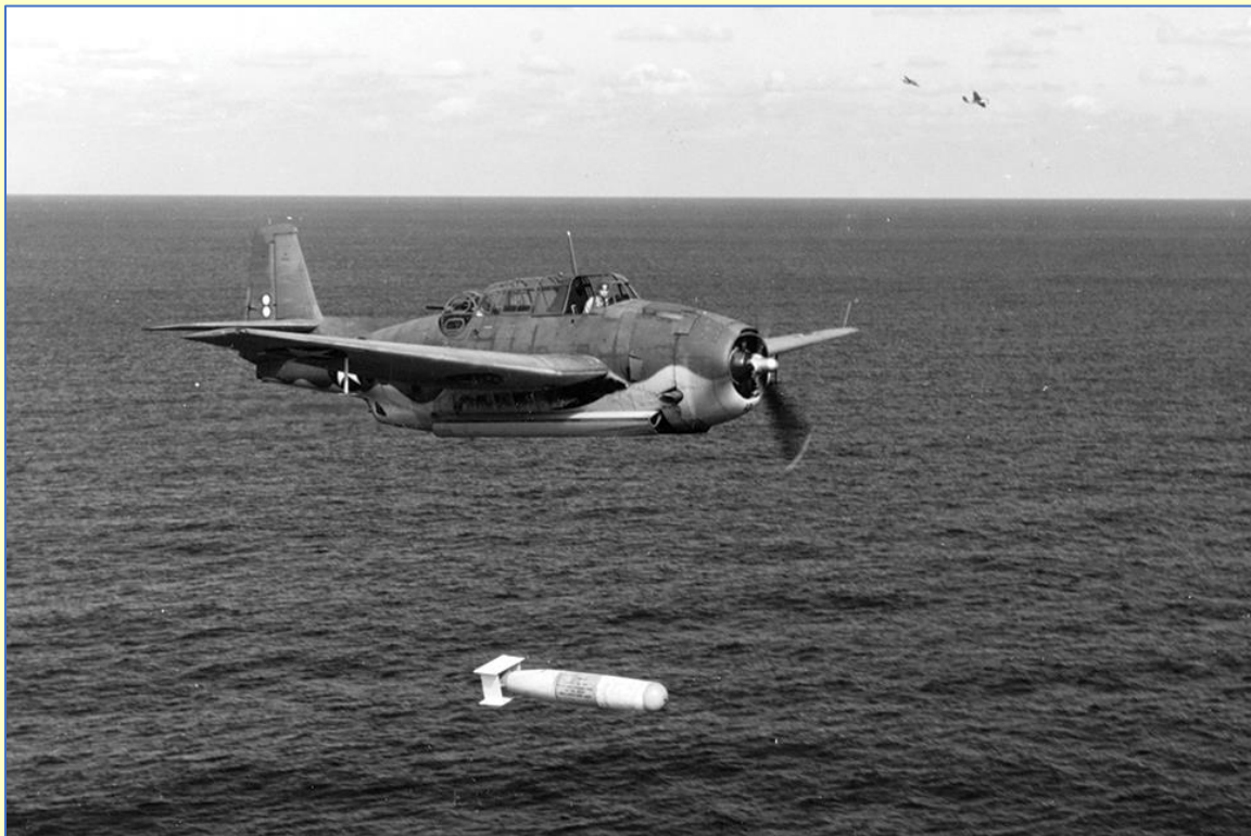
A TBF drops a Mark 13 during practice run in 1943. Note the "box-like" wooden stabilizer at the rear of the torpedo.
